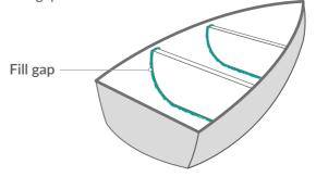
With the fillet tool at a 90° angle to the joint, form a fillet and remove excess material, which can be reused.
